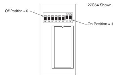
Figure 3.1 Channel DIP Switch Setting
