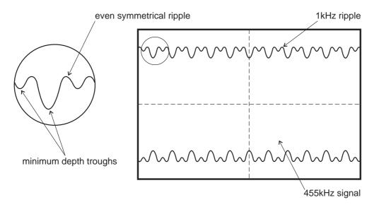
Figure 3.3 455kHz Signal With Even 1kHz Ripple
