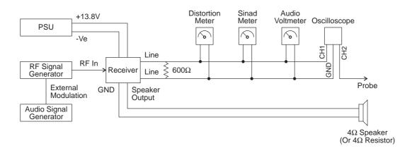
Figure 3.2 Test Equipment Set-up
